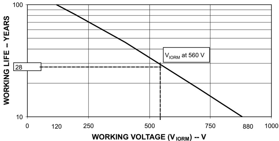
Figure 20. Time Dependent Dielectric Breakdown Test Results
