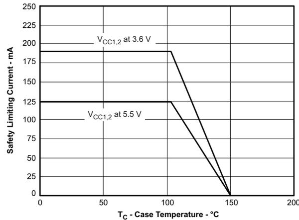
Figure 5. SOIC-8  $\theta_{JC}$  THERMAL DERATING CURVE per IEC 60747-5-2
